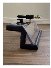
To guarantee the integrity of Keel Coolers, rigorous nondestructive testing inspection methods like Vacuum Box Testing are employed to detect defects in welded joints. This process ensures that the Keel Cooler is free from defects that could compromise its effectiveness, enabling it to maintain optimal engine temperatures and contribute to the overall efficiency and safety of the vessel during its operations at sea.
